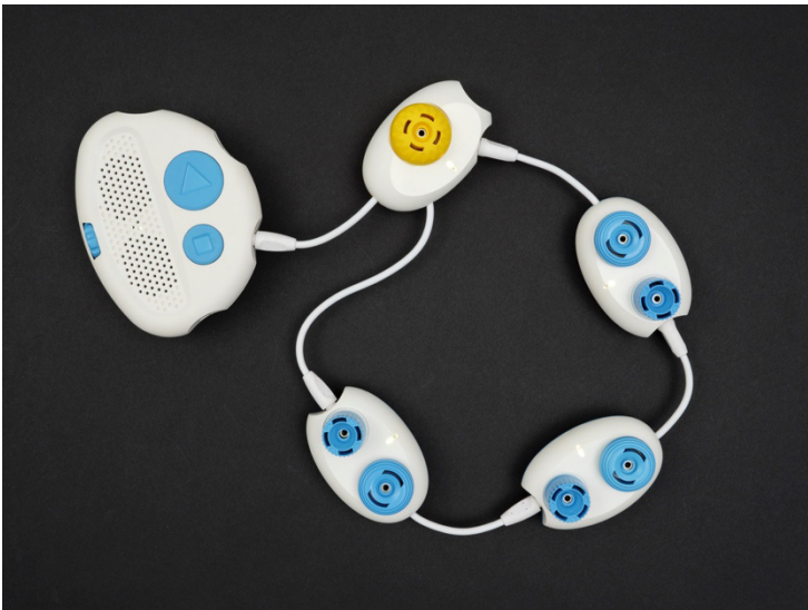
[Figure Caption:] At the top is a screenshot of the Code Jumper app with a program in Thread 3. Under Thread 3 Numbers, the commands read, LOOP 4 times, PLAY One for 1 times speed, PLAY Two for 1 times speed, PLAY Three for 1 times speed, END LOOP; the commands are followed by End Thread. Below the screenshot is a photo of the Code Jumper kit containing three Play pods and a Loop pod. The Loop pod is connected directly to the Hub at Port 2 by its shorter wire. The Play pods are connected, one after the other, to the Loop pod’s lower-right port and the Loop pod’s longer wire.
